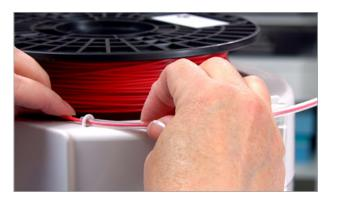
Once you've got a couple inches poking out the end of the clear filament tube, press it into the hole until it stops. You do not need to push the lever. This positions the filament right up against the gear of the feed motor.
