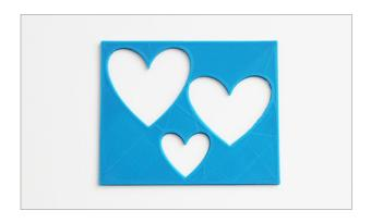
The Stencil choice takes the design and makes holes in a flat plate to create a stencil.
