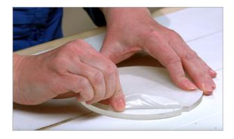
To remove the platform tape, simply peel it off like a piece of tape. Then take a new piece, line it up with the notch on the platform with the backing still in place. Peel away the backing of the lower half of the platform tape while holding the top half in place. Smooth the bottom half down with the included spatula tool, and then peel away the backing of the top half. Smooth down the remaining half to finish the application.
