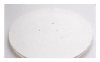
Scratches, holes, and tears in the platform tape will cause flaws to be carried through your 3D prints. The solution for this is to replace the platform tape. Try to smooth out any bubbles that may appear as you remove your prints from the platform tape because bubbles will affect prints as well.
