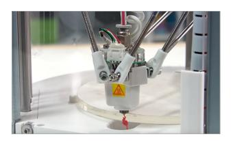
Insert the guide tube into the loading hole after the filament has finished loading. You don't need to press the lever at all in this process.
