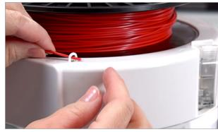
Push the filament through the small eye loop on the top of the Alta, and then slide it through the clear filament guide tube.
