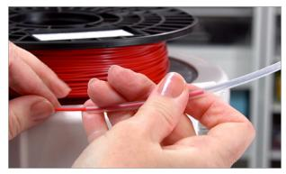
Put the top end of the guide tube through the loop so the filament doesn't wear away the loop as it moves.
