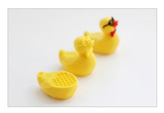
The density of infill changes with standard, draft, or high quality. Draft quality leaves bigger gaps in the infill, High quality has a denser infill, and Standard is in between.
