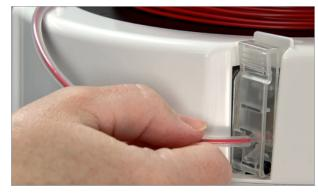
To unload the filament in order to store it or switch colors, use the same filament button on the 3D Print Tab and follow the instructions to unload the filament. The print head on the Alta will be heated, extrude a little filament, and automatically unload the filament.
